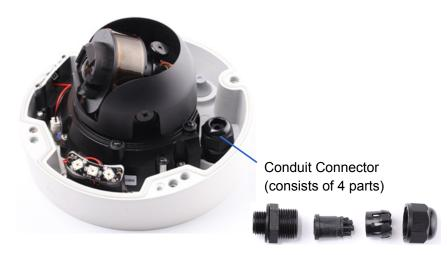
• Every plug has its designated cable. Only thread the assigned cable to the corresponding hole.
