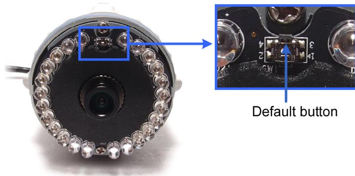
4. Release the **default** button. When the process of loading default settings is completed, the camera reboots automatically.
