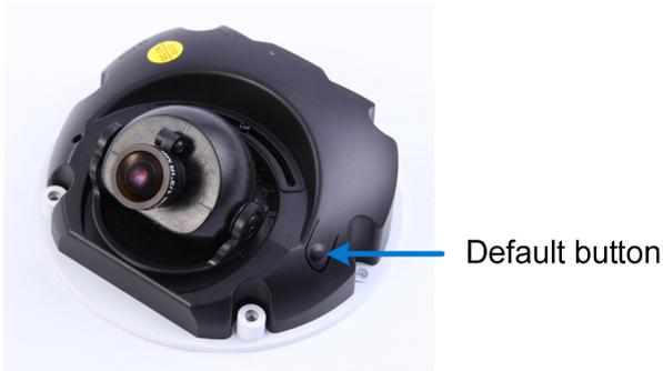
3. Release the **default** button when the **status LED** blinks. This shall take about 8 seconds.
