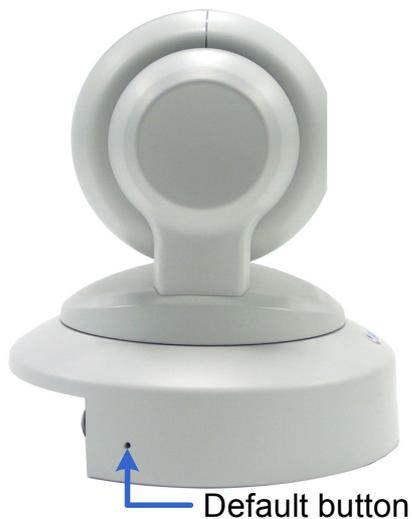
3. Release the **default** button when the **status LED** blinks. This shall take about 8 seconds.
