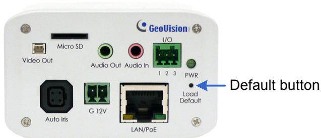
3. Release the **default** button when the **status LED** blinks. This shall take about 8 seconds.
