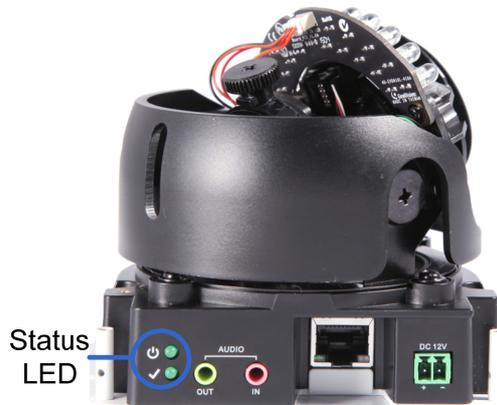
4. When the **status LED** fades, the process of loading default settings is completed and the camera reboots automatically
