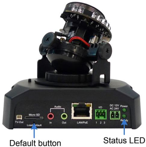
3. Release the **default** button when the **status LED** blinks. This shall take about 8 seconds.
