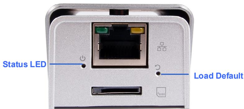
3. Release the **default** button when the **status LED** blinks. This shall take about 8 seconds.
